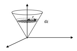
$$z_{G} = \frac{\int_{0}^{h} \sigma \, \pi \left(\frac{R}{h}\right)^{2} z^{3} dz}{\int_{0}^{h} \sigma \, \pi \left(\frac{R}{h}\right)^{2} z^{2} dz} = \frac{\left[\frac{z^{4}}{4}\right]_{0}^{h}}{\left[\frac{z^{3}}{3}\right]_{0}^{h}} = \frac{3}{4}h$$
