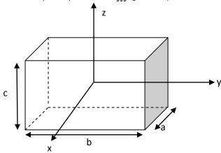
$$A = \rho \int_{-\frac{b}{2}}^{\frac{b}{2}} y^{2} dy \int_{-\frac{a}{2}}^{\frac{a}{2}} dx \int_{-\frac{c}{2}}^{\frac{c}{2}} dz + \rho \int_{-\frac{b}{2}}^{\frac{b}{2}} dy \int_{-\frac{a}{2}}^{\frac{a}{2}} dx \int_{-\frac{c}{2}}^{\frac{c}{2}} z^{2} dz = \frac{\rho}{12} \ abc \ (b^{2} + c^{2}) = \frac{m}{12} (b^{2} + c^{2})$$
