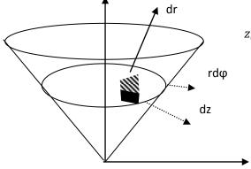
$$z_{G} = \frac{\iiint z dm}{\iiint dm} = \frac{\int_{0}^{h} z \left[ \int_{0}^{ztg\alpha} r \, dr \right] dz \int_{0}^{2\pi} d\varphi}{\int_{0}^{h} \left[ \int_{0}^{ztg\alpha} r \, dr \right] dz \int_{0}^{2\pi} d\varphi} = \frac{3}{4} h$$
