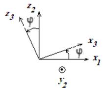
$$\Rightarrow \vec{G} = \begin{pmatrix} G_{x3} \\ G_{y3} \\ G_{z3} \end{pmatrix}_{R_3} = \begin{pmatrix} g \cos \theta \sin \varphi - R \ddot{\psi} \cos \varphi + R \dot{\psi}^2 \sin \theta \sin \varphi \\ g \sin \theta - R \dot{\psi}^2 \cos \theta \\ g \cos \theta \cos \varphi + R \ddot{\psi} \sin \varphi + R \dot{\psi}^2 \sin \theta \cos \varphi \end{pmatrix}_{R_3}$$
